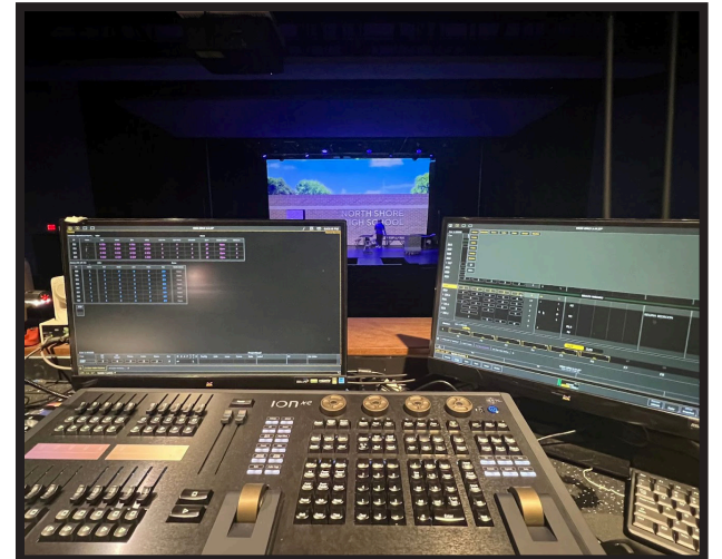
INSIDE THE BOX: Isha Patel ’24 controls the lighting on an Ion Xe panel from inside the box. (Photo Credit: Isha Patel ’24)
